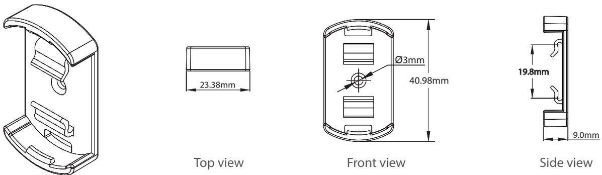
Tolerance for dimensions =  $\pm 2.5\text{mm}$
