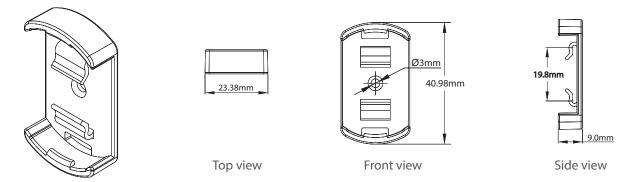
Tolerance for dimensions =  $\pm 2.5$ mm
