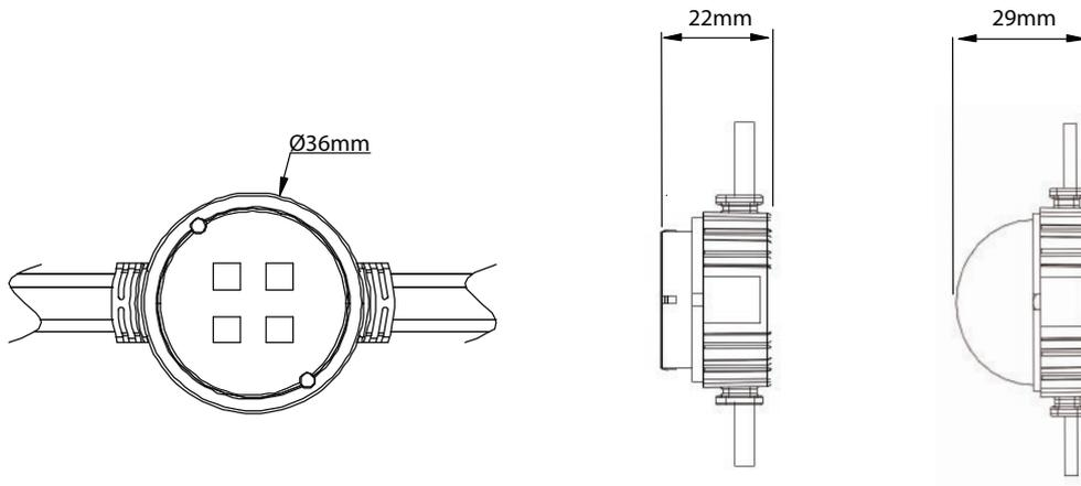
Tolerance for dimension =  $\pm 2.5\text{mm}$
