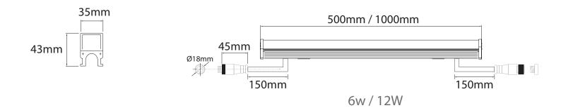
Tolerance for dimensions =  $\pm 2.5$ mm
