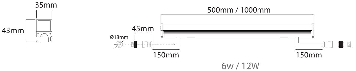
Tolerance for dimensions =  $\pm 2.5\text{mm}$
